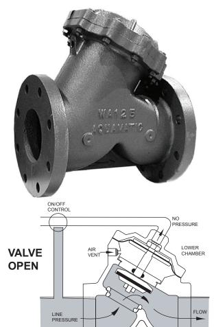
**Full Open Operation** When closing pressure, in upper chamber, is relieved by venting the pilot line, the valve opens, positively, by line pressure on the disc.
