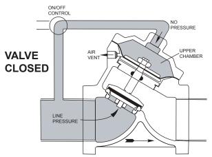
**Drip-Tight Closing** Closure is obtained by directing line pressure or equivilent independent pressure into the upper chamber. This pressure on the large diaphragm area causes the valve
